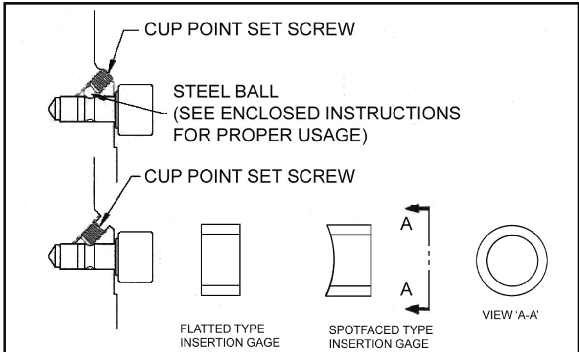
The H9 thru H32 (.287" thru 1.00" diameter) Cam Followers require a Steel Ball/Set Screw and an insertion gage for installation. The steel ball/set screw is used to anchor the cam followers to the follower wheel and the insertion gage kit is used to insure proper installation. The new cam followers need to be pressed onto the follower wheel to the position prescribed by the gage (if they are pressed in too far, they will not turn freely).
